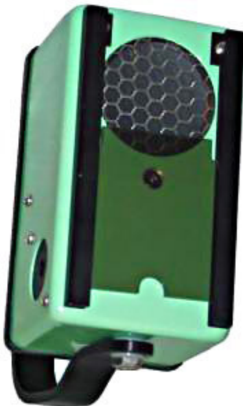
Bottom view of TBM-3SR showing sliding beta shield.
