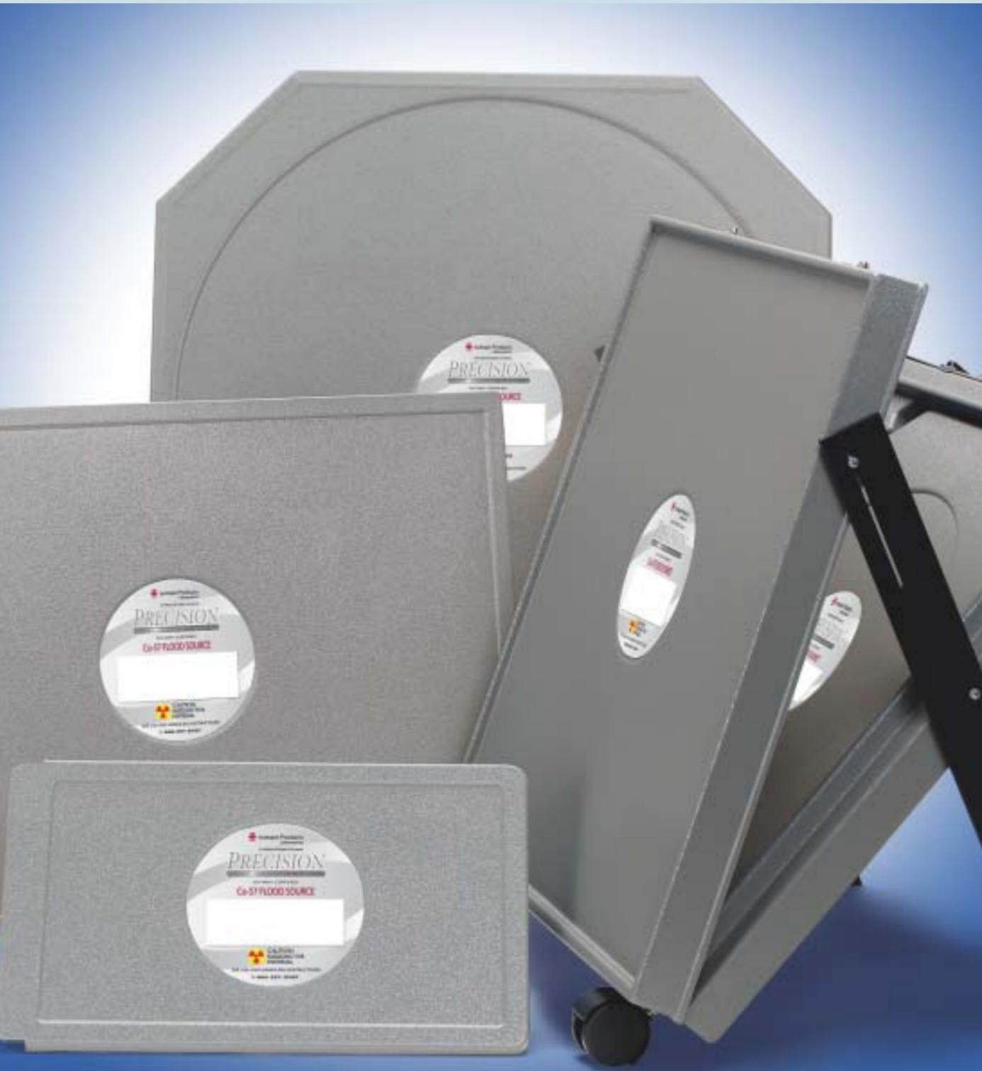
The Isotope Products Laboratories' Co-57 Flood Source provides a uniform field of radiation for evaluation of Nuclear Medicine gamma camera performance, allowing detection and correction of any camera malfunction prior to diagnostic use. The useful life of the Co-57 flood source is approximately 2 years. The Co-57 flood sources are available in a variety of circular and rectangular dimensions, with activities to meet the standards established by the manufacturers of the gamma cameras.
