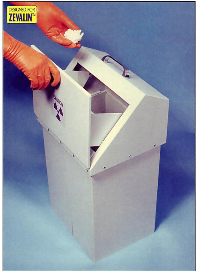
This Shielded Waste Container is used in facilities that generate low-energy beta and gamma radiation waste. The interior of the container is constructed of .063" aluminum (1.6 mm) and .25" lead (6 mm). The shielding combination attenuates gamma radiation, beta radiation and errant Bremsstrahlung.
