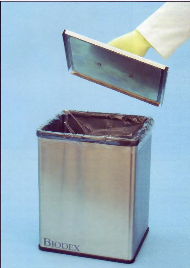
The Shielded Waste Container is a must for any facility that generates low-energy gamma radiation waste. Constructed entirely of 18-gauge stainless steel, and lined with .125" (3 mm) lead, this 20 quart (18.9 liter) capacity container can be placed on the floor or counter. Simply lift off the shielded cover for quick disposal of waste. Plastic liners make it easy to transfer waste to decay or disposal site once the container is filled.
